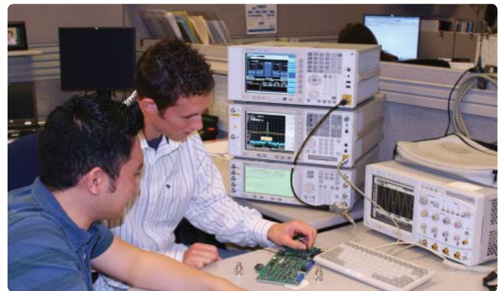
Engineers Michael Wohlert and Angelo Umali using Agilent spectrum analyzers to measure a circuit
